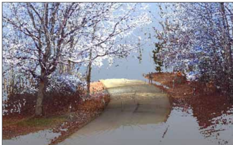
Figure 8 - 3D scan data of a curved roadway with visibility obstructions
