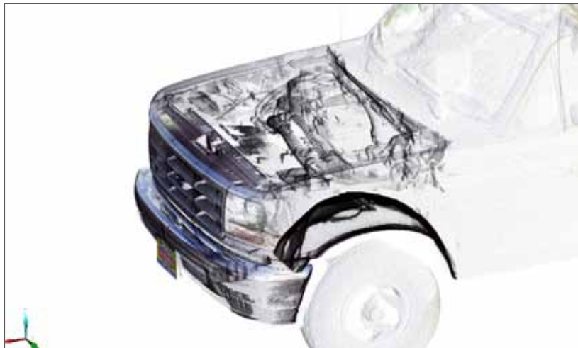
Figure 11 - 3D scan data with vehicle components visible
